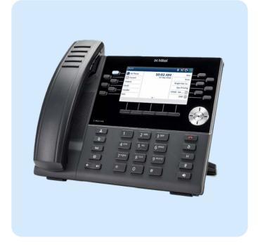
The 6930w's first-of-its-kind PCLink feature turns your phone into a high quality audio device for PC based video collaboration. PCLink enables seamless handling of both phone calls and PC audio through a single easy-to-use device. By connecting the phone to your favorite video collaboration solution you
